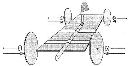
4. Blow up the balloon through the straw. Place string around partially filled balloon. Continue inflating until the circumference of the balloon is the same size as the circle of string. Squeeze the end of the straw. Place the car on the floor and let it go!
